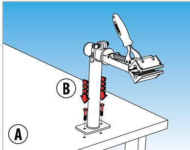
**When mounting swiveling vice jaw on the workbench (A), always mount like shown above. Mount jaw with two screws (B) that are included.** • Vpenjalno glavno privijemo na delovni pult (A) s pomočjo dveh priloženih lesnih vijakov (B) kot prikazuje slika.
