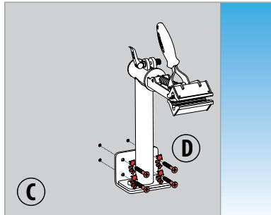
**When mounting swiveling vice jaw to the wall, always mount plate and jaw like shown above. Screw vice jaw with four screws to the wall.** • Vpenjalno glavo privijemo na zid (C) s pomočjo štirih priloženih vijakov (D) kot prikazuje slika.
